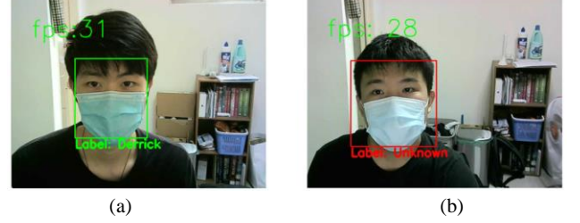
Fig. 6 Results of identification, (a)enrolled user identification, (b)unenrolled user identification.
